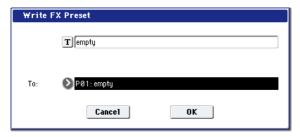
2. Press the text edit button to open the text edit dialog box, and enter a name for the effect preset.
