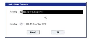
1. If you want to load a wave sequence other than the selected wave sequence, use "Wave Sequence" (the upper line) to re-select the wave sequence to be loaded.
