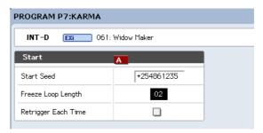
Note: "Seed" is the source data from which the randomizations are created. The "Seed" of the phrase being looped is automatically set internally within the KARMA Module as the "Start Seed." The "Start Seed" is used each time the GE is triggered. This means that each time you trigger the GE, a specific "Seed" is always used to generate the phrase.
