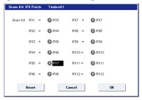
Use the **Drum Kit IFX Patch** page menu command if you want the drum program to use effects other than timbres 2 and 3. Choose **Drum Kit IFX Patch** from the page menu, and temporarily send the drum kit IFX1 to IFX3, IFX2 to IFX4, IFX3 to IFX5, IFX4 to IFX6, and IFX5 to IFX7 (Fig. 2–2d). Executing with these settings will temporarily change the effects to which the drum kit is being sent (Fig. 2–2e).
