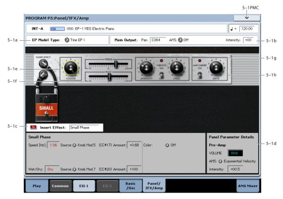
These parameters apply when one of the Tine pianos is selected as the **EP Model Type**.
