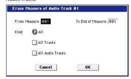
3. In From Measure select the first measure to be erased, and in To End of Measure select the last measure to be
