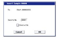
3. To Start will indicate the starting address at which the data will be inserted.
