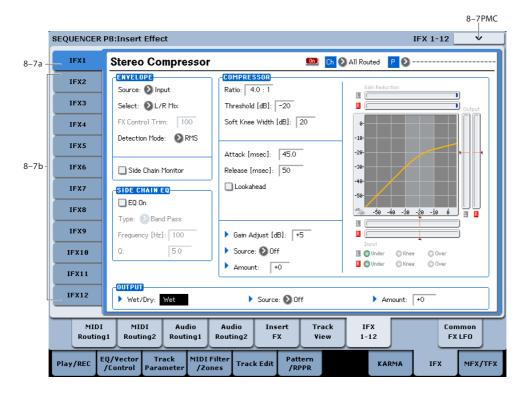
This page lets you edit the detailed parameters of the twelve insert effect s. Use the tabs at left to select IFX1 through IFX12.
