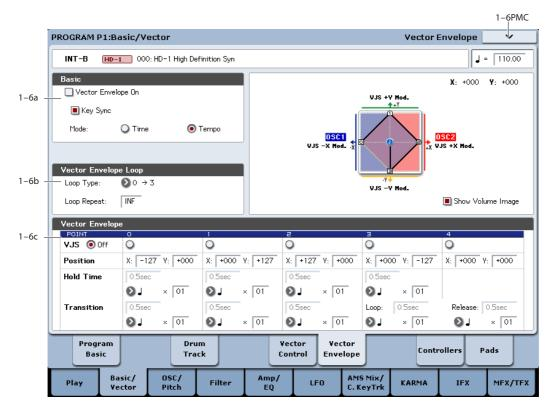
The Vector Envelope works together with the Vector Joystick to control the Vector position. It's also special because it's the only programmable modulation source which lets you modulate both Program and Effects parameters.
