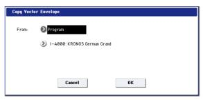
2. Use the "From" field to select the mode, bank, and number of the desired copy-source. You can press a BANK key to select the desired bank.
