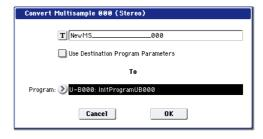
3. Press the text edit button to open the text edit dialog box, and set the Program name as desired (up to 24 characters).
