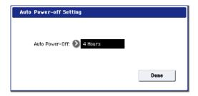
2. Press the "Auto Power-off" popup button to select the length of idle time after which the power will turn off. If you don't want the power to turn off automatically, set this to Disabled.
