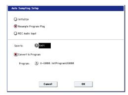
1. Use "Save to" to select either RAM or DISK as the destination to which the resampled data will be
