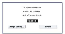
If you want to continue using the system, press the keyboard, a button, or some part of the display such as the Extend button. The Auto power-off function will be reset. If the specified length of time again elapses with no user input, the
