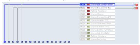
Example: Inserting a separate IFX into each timbre, and then inserting an IFX at the final stage
