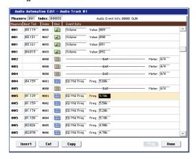
3. Measure and Index located in the top line of the dialog box show the measure for editing and the index number of an event within that measure; this event is shown at the top of the list of events.
