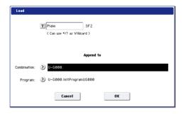
1. Use "Append to: Combination" to specify the destination bank and number of the combination that will be created by the convert-load operation.
