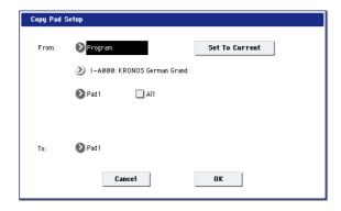
2. Use the "From" field to select the mode, bank, and number of the desired copy-source. You can also select Banks via the front-panel BANK SELECT buttons.
