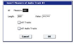
3. In "At Measure," specify the measure location at which the data will be inserted. (The measure you specified in Track Edit page From Measure will be set as a default.)
