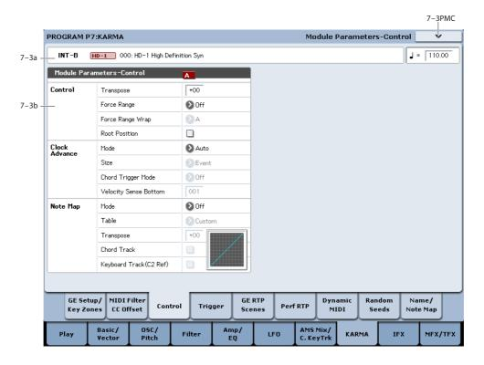
Here you can set KARMA Module Control parameters. Note that in Program mode, you can use one KARMA Module (Module A).
