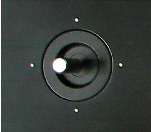
You can alter the sound mix of a Preset by turning the Joystick in all directions and from one point to the next in any speed. Using this function can help to get more real time modification effects into your sounds.
