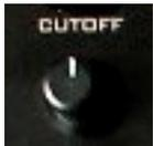
Turning the Knob to the left will reduce the amount of high frequencies and the tone will be soft and a dull. Using this effect during playing performance is typical for many music styles and is very interesting too for Arpeggios. The Filter Cutoff works in combination with the next Knob 2.
